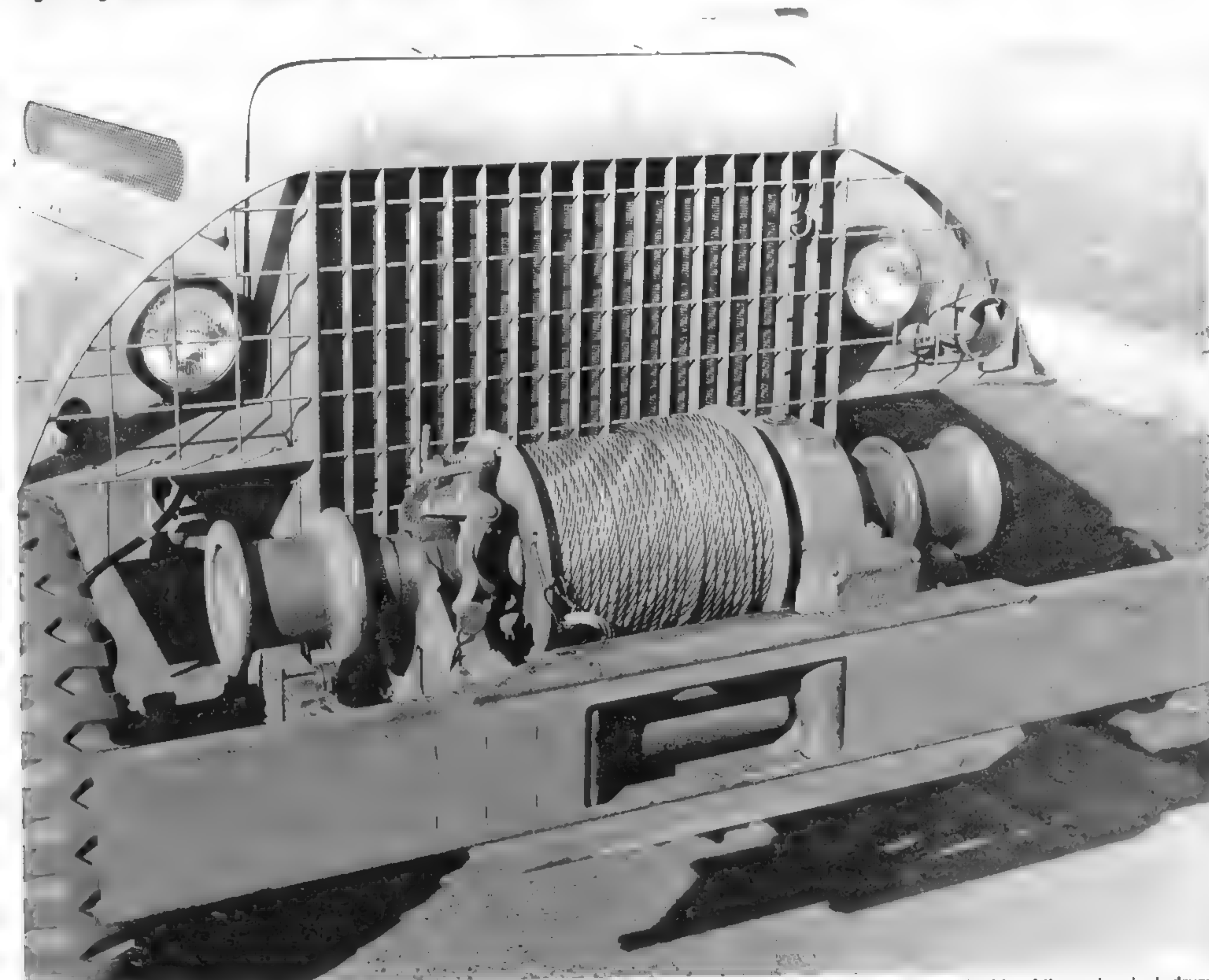
The front-mounted winch came on many of the 6-ton vehicles. The trucks were equipped with a capstan drum on each side of the main winch drum. (White Motor Company photo)
